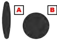
Fig. 5: Normal spray image: Flat jet (A) and round jet (B)
