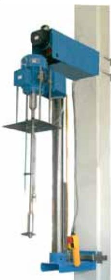
Wall mount with electric cable winch and caustic solution blender
