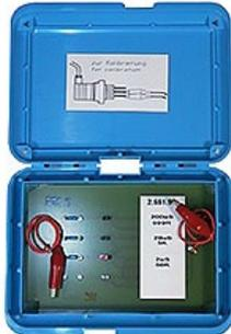
**Calibration box for conductivity measurement (conductive)**
