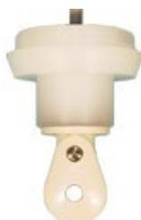
**Conductivity measuring probe as aforementioned, with adapter**
