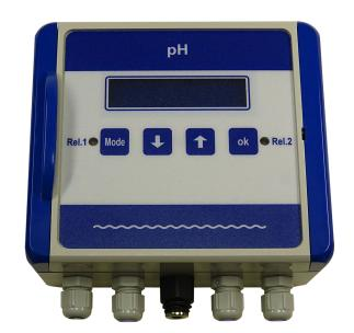
The EcoTrans II measurement transmitter records measurements in a range from pH 0 to pH 14 and converts these into a 4 - 20 mA standard signal (pH 0 = 4 mA, pH 14 = 20 mA).
