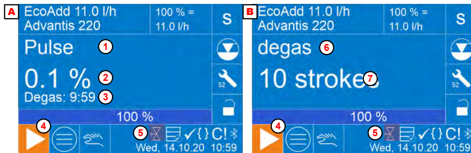
Fig. 6: Degassing, venting process
