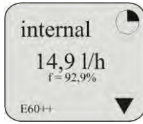
Fig. 10.30 Display in the operating display with an active metering controller: Downward metering divergence
