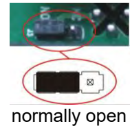
Fig. 7.26 normally open contact
