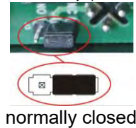
Fig. 7.27 normally closed contact
