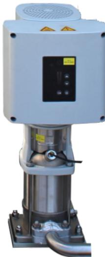
Grundfos E-pumps are fitted with frequency-controlled permanent-magnet motors for single-phase or three-phase mains connection. The pumps have a built-in PI controller and can be set for an external sensor enabling the control of the following parameters:
