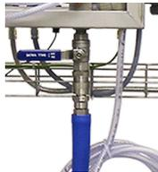
5. ▶ Open the valve under the Foamatic satellite.
