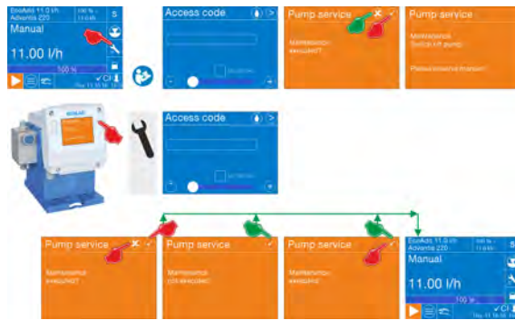
Fig. 23: Put the pump in the maintenance mode when an access code is being used
