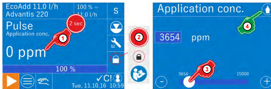
Fig. 41: [Change Pulse] [Concentration] [ppm]at operating level
