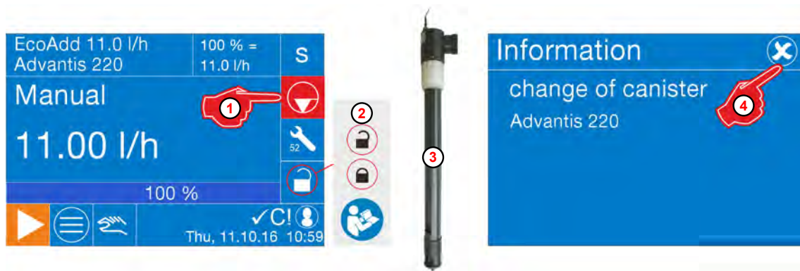
Fig. 96: Empty signal: Change container
