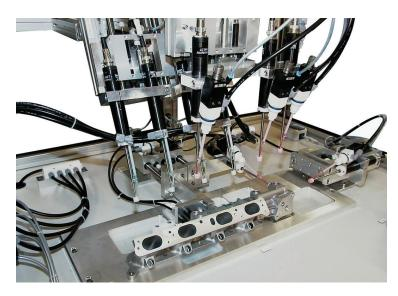
Fully automatic metering system for circular dispensing of oil or adhesives in several internal threads / bore holes
