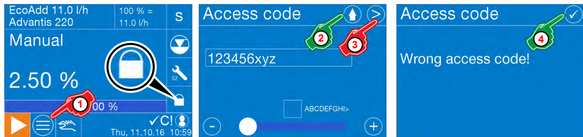
Fig. 54: Incorrect password input
