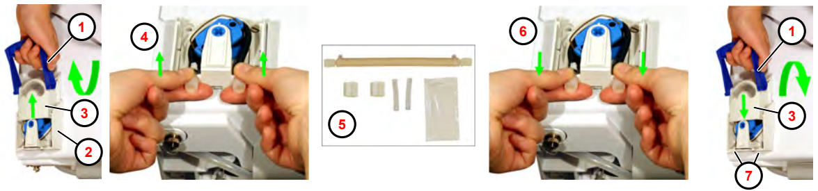
Fig. 25: Replacing the peristaltic hose
